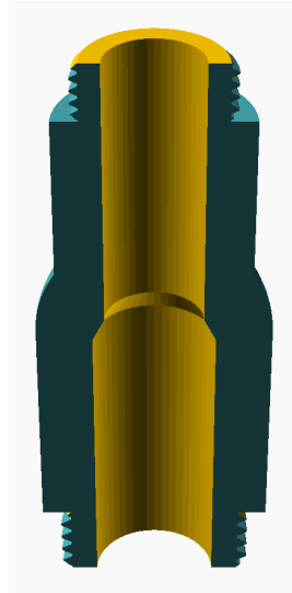
Figure 44: Reducer, default variant, cutaway (BOSL2 BACK) showing the bore.
