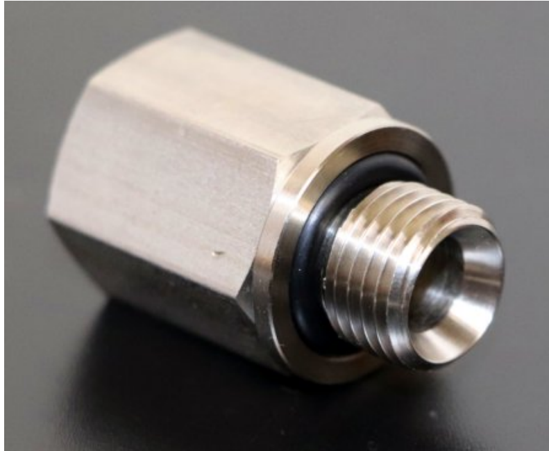
Figure 1: BSPP male straight-thread fitting with a hex flange and a captive O-ring seated against the flange’s underside. The thread is parallel along its length (constant outside diameter); the seal is made on assembly when the O-ring is compressed between the male flange and the female face — the threads themselves are not the sealing surface. Photograph by Kees08, CC BY-SA 4.0, via Wikimedia Commons. See also Sources and Attributions .
